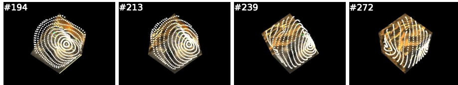
Fig. 5. Selected frames from the CUBE1 sequence. Notice, how TMAGIC learns the new face of the cube. #194: unknown shape, the surface is smoothed over. #213: first features detected, shape roughly estimated. #239: more features identified, shape refined. #272: Final state, model in agreement with the object.
